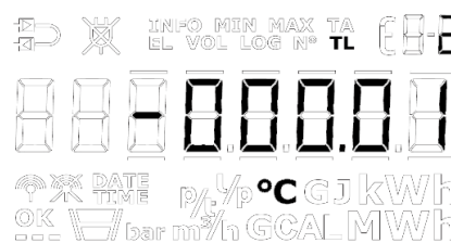
Figure 22 - Setting up negative TL2 in "SETUP loop", the - will be flashing when on the sign position and stay on when moving to another decimal.
