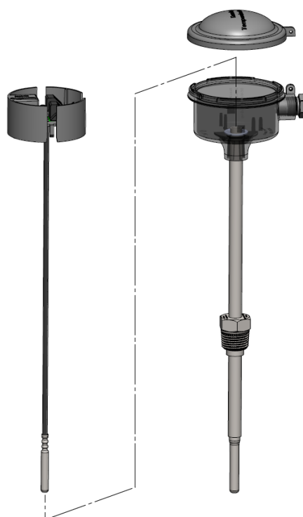
Figure 13: A \varnothing 5.8 mm pocket sensor with connection head can, for example, be mounted in a tee as shown in Figure 14.
