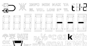
Display of differential temperature t1-t2 in case of temperature sensor error
